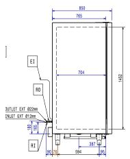
Drain Electrical inlet (power) RΩ Refrigerant Outlet
